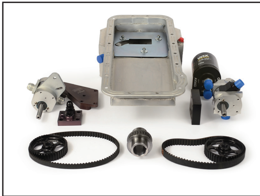
Shown is Ford FE external wet sump with both left and right-side mounts.
